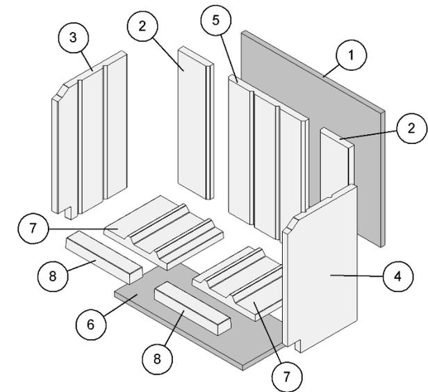
Figure 4 Refractory Bricks and Insulation Panels
