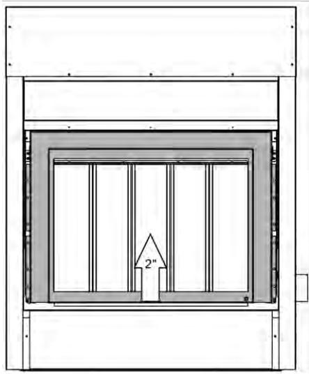
2. Unlatch the assembly on both sides.
