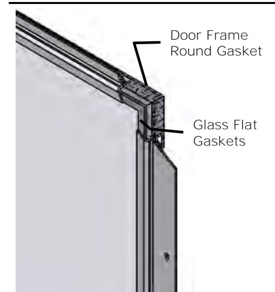
Figure 3 Top Right Corner of Glass Frame
