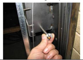
At the bottom outside corners of the guillotine door frame, on each side of the door there is a threaded oval connector. Unscrew both connectors and leave them unscrewed. Do not unhook the cable from the door yet.
