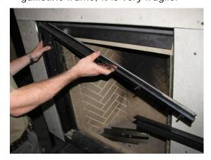
You can stop here if you only want to change the stainless steel gasket located at the top of the guillotine frame.
