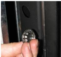
Using either a flat screw driver or bare hands, remove the decorative cover at the top of the guillotine frame. It is pressure fitted, pull down and out.
